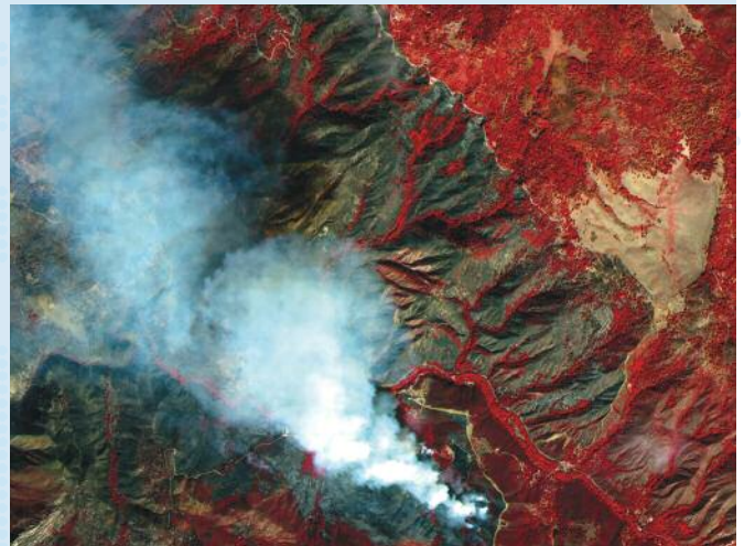
Forest fires observed (1m resolution) by KOMPSAT-2 on 28 October 2007 over California, USA. The burnt area shown in dark blue, vegetation in red and the smoke of active fires in light blue and white. ©KARI 2007
