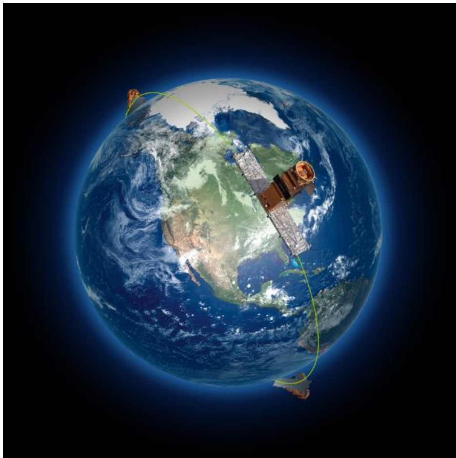
Canada's new generation of Earth observation satellites, the RCM consists of three satellites, evenly spaced on the same orbital plane at an altitude of 600 km. (Credit: Canadian Space Agency)
